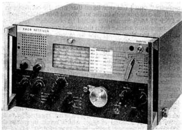
The Redifon R408 all-transistor communications receiver covers 13 kc/s to 28 Mc/s without a break.
